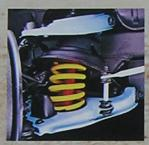
Independent front suspension. Each front wheel rolls over bumps independently. Jolts and jars are absorbed by big coil springs and shock absorbers. Front stabilizer bar reduces roll and sway. Long 104.3-inch wheelbase spaces out and dampens down bumps for a smooth ride.
