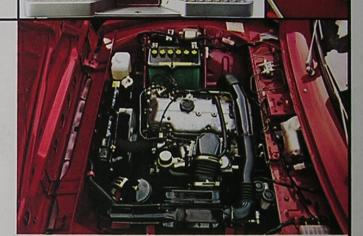
Big 4-cylinder, 1800-cc. displacement engine provides plenty of pep and power. Construction features include full-circle water jackets, cast iron cylinder block, cast aluminum cylinder head and valve cover, full pressure lubrication and large capacity oil pan. Standard four-on-the-floor transmission is synchronized in all forward speeds. Short-throw design gives fast, easy shifting.
