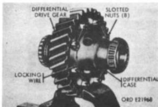
Figure 87. Removal of differential slotted nuts and bolts
