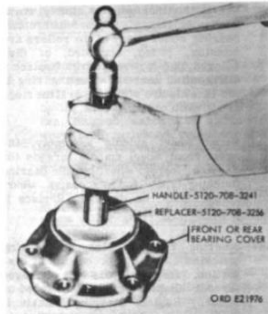
Figure 96. Installing front and rear bearing cover oil seals
